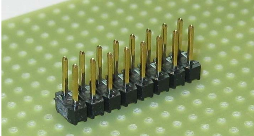
DIL (Dual In-Line) Header Installed On A Solderable PC Board
